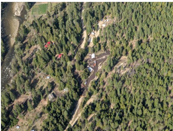
Photo 5. Debris flow deposit
